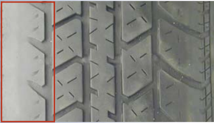
Uneven tread wear can be caused by improper wheel alignment or a tire imbalance.
