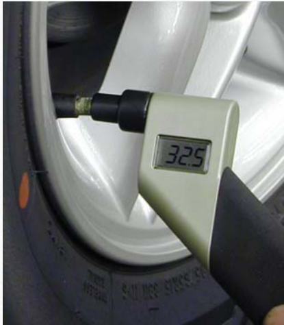
Tire pressure gauges sold by automotive supply stores are generally more accurate than those on gas station air pumps.
