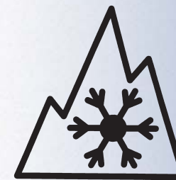
Tires designed for use in snowy weather are marked with the peaked mountain with snowflake symbol.
